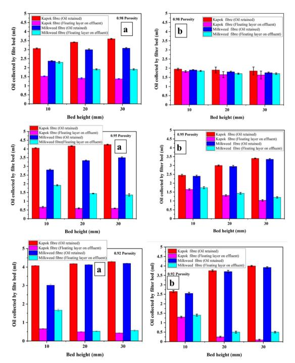
Fig. 5 Oil retained by kapok and milk weed filter beds of different heights, bed porosity with oil droplet size: (a) D50<sub>in</sub> 5 μm and (b) D50<sub>in</sub> 2 μm.
