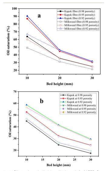
Fig. 4 Oil saturation vs. bed height and bed porosity for (a) D50  $_{in}$  5  $\mu m$  and (b) D50  $_{in}$  2  $\mu m$ .
