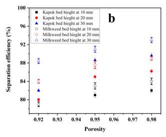
Fig. 2 Kapok and milkweed filter bed height, bed porosity on oil separation efficiency for (a)  $D50_{in}$  5  $\mu m$  and (b)  $D50_{in}$  2  $\mu m$ .
