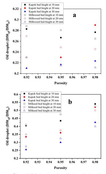
Fig. 3 Dispersed oil droplet size ratio and bed porosity interaction with (a) D50 $_{in}$  5  $\mu m$  and (b) D50 $_{in}$  2  $\mu m$ .
