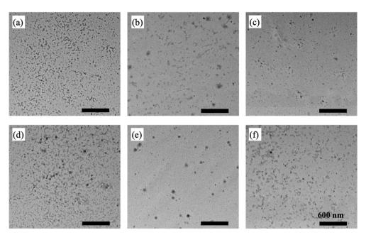
Fig. 5 Transmission electron microscopy (TEM) of SPEEK(72%) containing (a) 5 mass%, (b)15 mass%, and (c) 25 mass% LMW lignin and (d) 5 mass%, (e) 15 mass%, and (f) 25 mass% HMW lignin. Note, the scale bar in each image is 600 nm.
