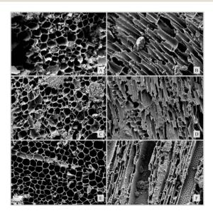
Fig. 1 SEM images of *Cannabis sativa* L. chemotype II stem-derived biochar produced at 400 °C (A and B), 600 °C (C and D), and 800 °C (E and F). Cross-sectional views are displayed on the left side, while longitudinal sections are shown on the right side.
