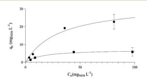
Fig. 3 Ammonia adsorption isotherms for C-400 (circles) and C-800 (squares). The fitting lines correspond to the Langmuir isotherm (with  $Q_0 = 32.6 \text{ mg}_{\text{NH4}} \text{ L}^{-1}, k_{\text{L}} = 0.032 \text{ L} \text{ mg}_{\text{NH4}}^{-1}, R^2 = 0.986 \text{ for C-400}$  and  $Q_0 = 7.1 \text{ mg}_{\text{NH4}} \text{ L}^{-1}, k_{\text{L}} = 0.065 \text{ L} \text{ mg}_{\text{NH4}}^{-1}, R^2 = 0.984, \text{ for C-800}.$
