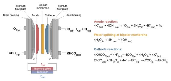
Fig. 1 A thermoelectrically-powered reactive carbon electrolyzer. Schematic of an exploded view of the zero-gap reactive carbon electrolyzer connected to the thermoelectric generator (not drawn to scale) used in this study and the accompanying electrochemical reactions at each component of the electrolyzer.
