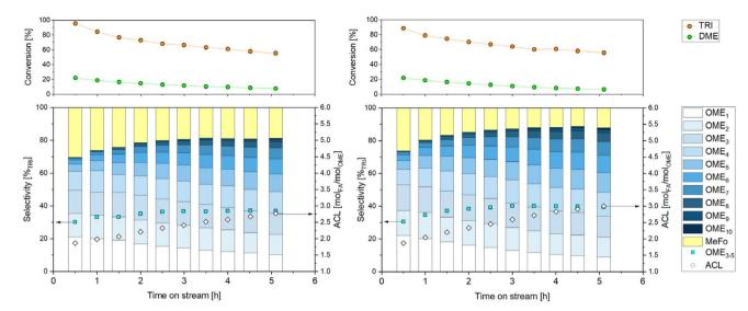
Fig. 5 Experimental results from continuous OME synthesis with KIT-Z80PU (left) and KIT-Z80AE (right) employing feed C1. Reaction conditions:  $T = 100 \, ^{\circ}\text{C}$ ,  $p = 40 \, \text{bar}$ .
