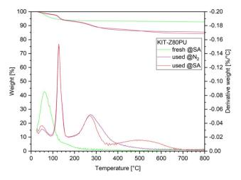
Fig. 8 TGA results for the fresh catalyst KIT-Z80PU and used in two consecutive runs with feed C2, measured under synthetic air ( $\alpha$ SA) and nitrogen ( $\alpha$ SA) atmosphere, respectively.
