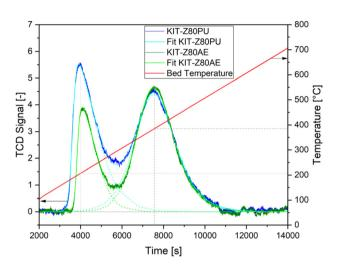
Fig. 4 NH<sub>3</sub>-TPD analysis for KIT-Z80PU (measurement: blue, fit: cyan) and KIT-Z80AE (measurement: olive, fit: green), catalyst bed temperature in red. Deconvolution in low (~200 °C) and high (~385 °C) temperature peak performed with OriginPro peak analysis.
