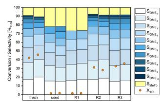
Fig. 10 Results of batch experiments employing fresh, used and regenerated KIT-Z80PU. Experimental conditions: T = 100 °C, t = 2 h, 2.6 wt%<sub>R</sub> catalyst, feed B1 (50 wt% *n*-dodecane).
