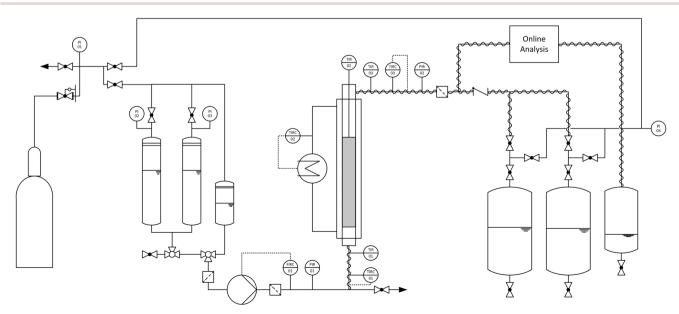
Fig. 1 Simplified flow diagram of the process module for continuous OME synthesis.
