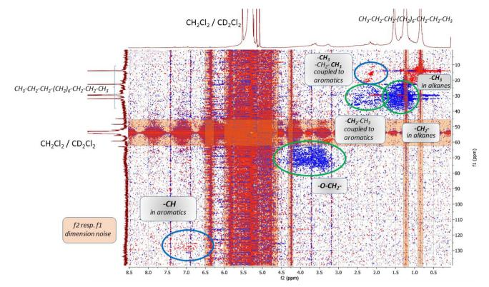
Fig. 13 2D <sup>13</sup>C, <sup>1</sup>H-correlated NMR spectrum (HSQC) of the organic extract of the soluble carbonaceous species, recorded with CD<sub>2</sub>Cl<sub>2</sub> (ca. 1:1 mixture)
