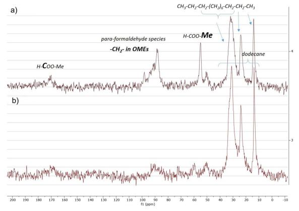
Fig. 11 <sup>13</sup>C MAS NMR spectra of (a) spent catalyst and (b) R1 (regenerated at 120 °C under N<sub>2</sub>).
