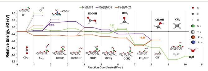
Fig. 7 Energy diagram for  $Ni@Ti_3$ ,  $Ru@Mo_2$ , and  $Fe@Mo_2$ . The diagram includes the pathways to methane (CH<sub>4</sub>) and methanol (CH<sub>3</sub>OH). On the bottom, the main intermediates are presented and match the curves above. On top, the final products, side products or intermediates are shown and match the thin curves below them, if applicable. The reaction coordinate number represents the number of PCET steps, except for adsorption and desorption steps.
