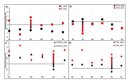
Fig. 5 Adsorption energies of: (a) H and (b)  $CO_2$  on a slab and SAC, for the six chosen transition metals. Similarly, desorption energies of: (c)  $CH_3OH$  and (d)  $CH_4$ . Arrows show the biggest difference between the slab and SAC for each sub-figure.
