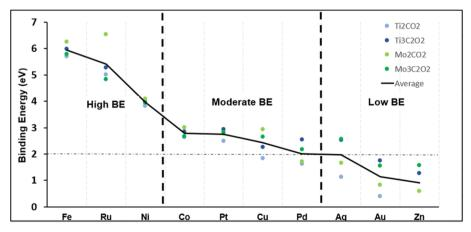
Fig. 2 Binding energy of single metals adsorbed on four different structures.
