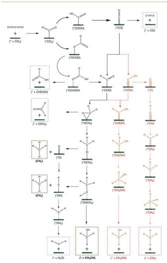
Fig. 3 Different pathways for the CO<sub>2</sub>RR leading to carbon monoxide, formic acid, methane, and methanol. Compounds with an asterisk \* are adsorbed species, while compounds with no asterisk are either reactants or desorbed products. Red pathways are deemed unfavourable on most catalysts. Species in dashed boxes are final products. Products in blue boxes are intermediate, unfavourable products. Products in green boxes are the targeted products in this study: methanol and methane.
