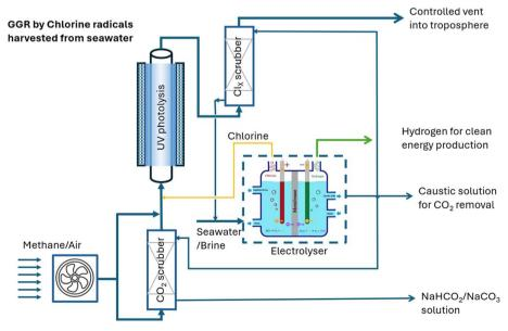
Fig. 4 The proposed integration of brine/seawater electrolysis and photolysis of Cl<sub>2</sub> gas for methane and CO<sub>2</sub> removal.
