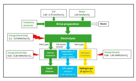
Fig. 5 Overview of the main materials flows and process of the chlor-alkali production using the diaphragm process.<sup>65</sup>
