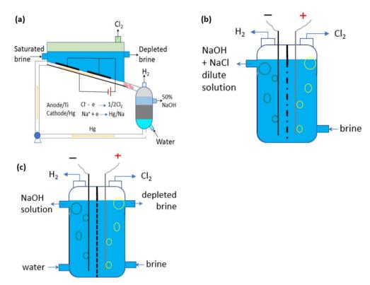
Fig. 3 Schematic methods for the industrial chlor-alkali process to produce Cl<sub>2</sub>: (a) mercury-based; (b) diaphragm; and (c) membrane methods. Adapted from.57
