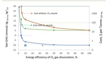
Fig. 6 Estimation of net GHG removal and cost with energy efficiency in Cl<sub>2</sub> gas dissociation. The hollow circle and the solid bar at the left bottom corner represent the net GHG removal when using clean energy from biomass, wind or nuclear sources.
