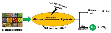
Fig. 7 A one-step approach using dark fermentation bacteria to produce biohydrogen; adapted from ref. 201.
