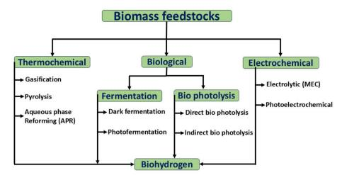
Fig. 4 The primary routes for the generation of biohydrogen derived from biomass
