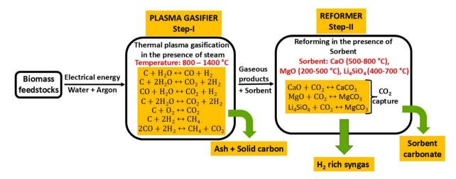
Fig. 5 Diagram depicting the suggested two-step process for sorption-enhanced gasification that includes CO<sub>2</sub> collection and the generation of clean energy adapted from ref. 104.
