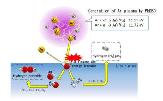
Fig. 1 Schematic diagram illustrating the mechanism of water decomposition *via* NgPCS, resulting in hydrogen (gas phase), and hydrogen peroxide (liquid phase) production. Water molecules are dissociated by the collision energy of noble gas plasma (argon: Ar).
