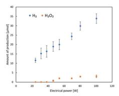
Fig. 3 Relationship between electrical power input and the amount of H<sub>2</sub> and H<sub>2</sub>O<sub>2</sub> generated via NgPCS.
