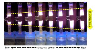
Fig. 4 Pictures showing argon plasma discharge at different electrical power inputs. At higher electrical power levels, the plasma extends to
