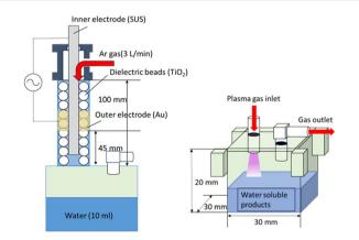
Fig. 2 Schematic diagram showing the experimental setup used for performing the NgPCS.
