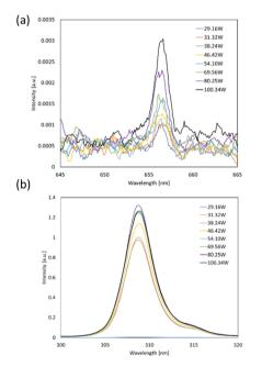
Fig. 7 Plasma emission spectra recorded at different electrical power inputs. Emission spectra corresponding to (a)  $H\alpha$  and (b) OH, resulting from water decomposition *via* NgPCS.
