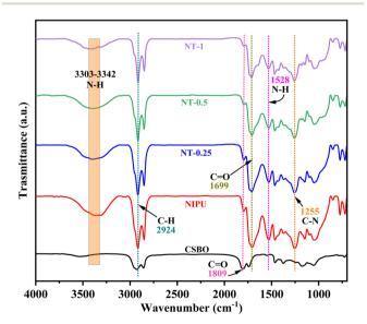
Fig. 1 ATR-FTIR spectra of NT-X composites
