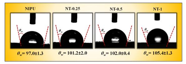
Fig. 8 Water contact angle (WCA) analysis of the prepared NIPU, NT-0.25, NT-0.5, and NT-1 composite films.
