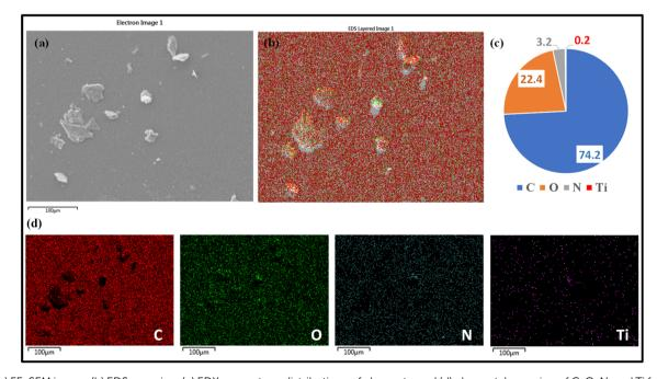
(a) FE-SEM image, (b) EDS mapping, (c) EDX percentage distributions of elements, and (d) elemental mapping of C, O, N, and Ti for the NT-Fig. 7 1 film.
