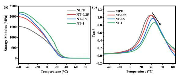
Fig. 4 DMTA curve of NT-X films: (a) storage modulus vs. temperature and (b)  $\tan \delta$  vs. temperature curves
