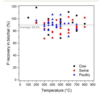
Fig. 5 Phosphorus recovery in biochars produced from cow (n = 15), swine (n = 25), and poultry manure (n = 25). The average value of 89.9% is calculated over all temperatures and manure types. Values are based on data from various sources. 47-50,56,57,59,65,68-70,124
