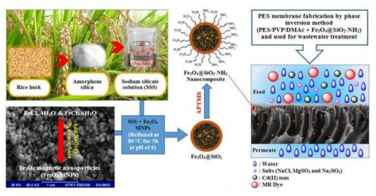
Graphical representation of the fabrication of Fe<sub>7</sub>O<sub>4</sub>@SiO<sub>2</sub>-NH<sub>2</sub>-embedded PES membrane and its waste water treatment application.<sup>40</sup>
