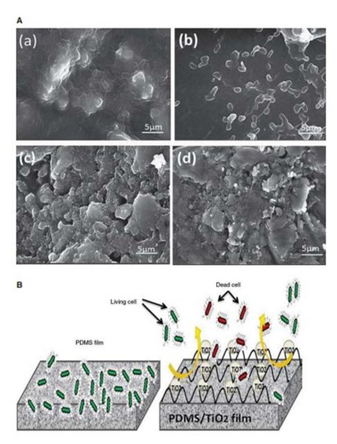
Fig. 7 (A) SEM images of the composite film at different concentrations of TiO<sub>2</sub>: (a) 0 wt%, (b) 7 wt%, (c) 10 wt%, and (d) 13 wt%. (B) Schematic of antibacterial mechanism of the composite film.47
