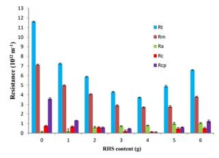
Fig. 9 Resistance,  $R_t$ : total;  $R_m$ : membrane;  $R_a$ : due to absorption;  $R_c$ : due to cake layer;  $R_{\rm cp}$ : due to cake polarization.<sup>54</sup>
