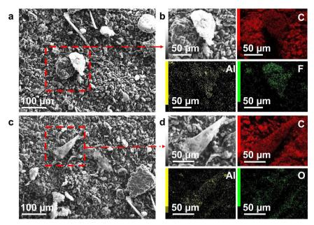
Fig. 2 SEM images of spent graphite anodes. (a and b) SEM-EDS mapping of Al foils detected in graphite. (c and d) SEM-EDS mapping of  $Al_2O_3$  particles detected in graphite.
