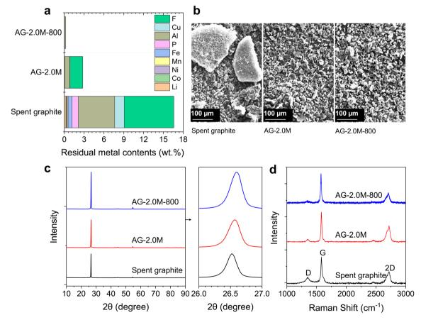
Fig. 5 Characterisation of recovered graphite. (a) Residual metal contents after optimized recycling processes. (b) SEM images. (c) XRD spectra. (d) Raman spectra. AG-2.0M: graphite recovered via 2 M H<sub>2</sub>SO<sub>4</sub> leaching. AG-2.0M-800: graphite recovered via 2 M H<sub>2</sub>SO<sub>4</sub> leaching followed by 800 °C pyrolysis.
