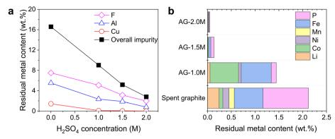
Fig. 3 Weight percentages of residual metals in spent graphite after secondary acid leaching. (a) Al, Cu, F and overall impurity contents as a function of acid concentration. (b) Other residual metal contents after leaching processes. AG-X samples, where X represents  $H_2SO_4$  concentration
