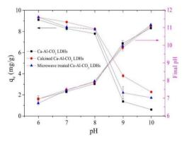
Fig. 10 Effect of initial pH on the F<sup>-</sup> removal by Ca-Al-CO<sub>3</sub> LDH and its modified products. (Initial  $F^- = 10 \text{ mg L}^{-1}$ , adsorbent dose = 1 g L<sup>-1</sup>,  $T=25\pm1$  °C, and  $q_{\rm e}$  is the equilibrium adsorption capacity).<sup>75</sup> Copyright 2020, Elsevier.
