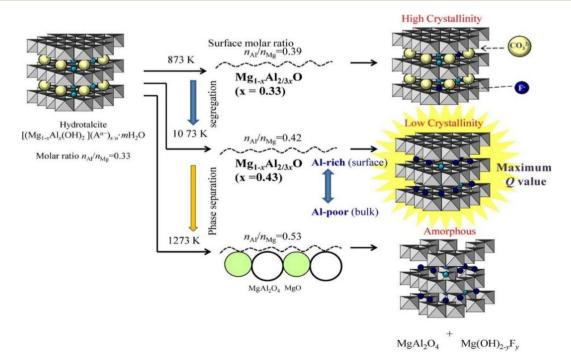
Fig. 6 Effect of calcination temperatures on the structure of LDH.<sup>67</sup> Copyright 2014. Elsevier
