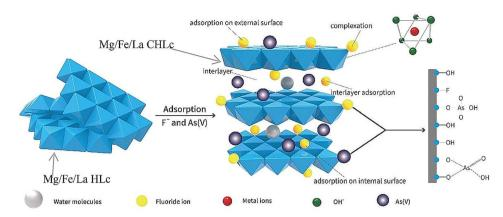
Fig. 18 MMO hydration mechanism for fluoride ion adsorption by MgFeLa-MMO.<sup>28</sup> Copyright 2018, American Chemical Society.
