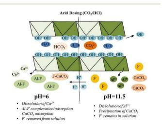
Fig. 16 Cationic complexation mechanism for the removal of fluoride ions by CaAl-LDH. 112 Copyright 2021, Elsevier.
