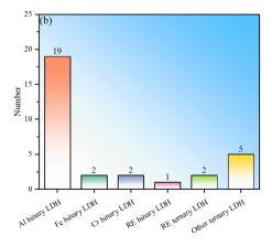
Fig. 1 Statistical histogram of intrinsic LDH fluoride ion removal agents. (a) Removal performance expressed as adsorption capacity and (b) the number of studies (Note: heterocoagulated composites or LDH derivative MMOs are not considered here, and only intrinsic LDH adsorption is compared. There are no error bars for rare element-based binary LDH because of the presence of only one study.).
