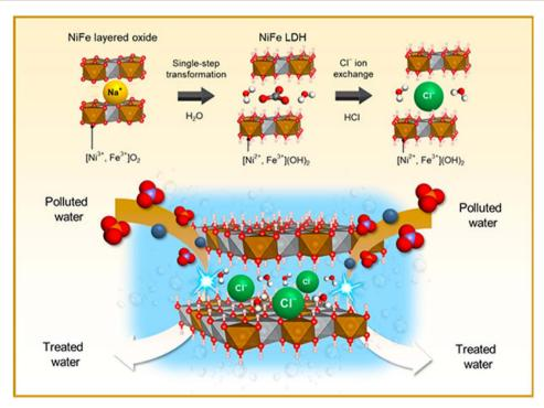
Fig. 5 Schematic diagram of the synthesis of NiFe-LDH with interlayer Cl ions.<sup>20</sup> Copyright 2021, American Chemical Society.
