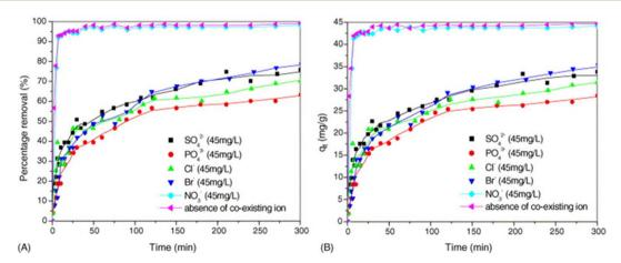
Fig. 14 Relationship between the percentage removal of fluoride and the adsorption time (A) and the adsorption loading of fluoride and the time (B), for various co-existing anions (V = 1.8 L, pH = 6.0, F<sup>-</sup> = 50 mg L<sup>-1</sup>, and adsorption mass = 2.0 g). Copyright 2006, Elsevier.
