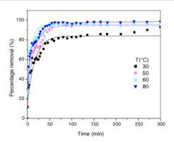
Fig. 12 Relationship between the percentage removal of fluoride ions and the time for various temperatures (V = 1.8 L, pH = 6.0, F<sup>-</sup> = 50 mg  $L^{-1}$ , and adsorbent mass = 2.0 g). <sup>13</sup> Copyright 2006, Elsevier.
