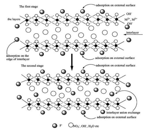
The anion exchange mechanism for the removal of fluoride ions by Mg<sub>2.5</sub>Ca<sub>0.5</sub>Al-NO<sub>3</sub>-LDH.<sup>38</sup> Copyright 2012, Elsevier.
