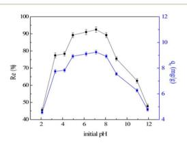
Fig. 11 Effect of initial pH (V = 50 mL,  $T = 25 \pm 1$  °C, C0 = 10 mg L<sup>-1</sup>,  $R_{\rm e}$  is the removal percentage and  $q_{\rm e}$  is the equilibrium adsorption capacity).64 Copyright 2016, John Wiley and Sons.
