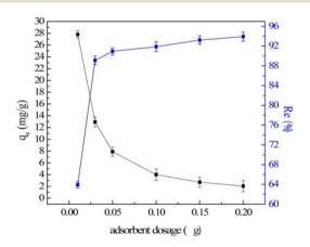
Fig. 13 Effect of adsorbent dosage ( $V=50~\rm mL;~T=25\pm1~^\circ C;~C_0=10~\rm mg~L;~q_e$  is the equilibrium adsorption capacity). <sup>64</sup> Copyright 2016, John Wiley and Sons.
