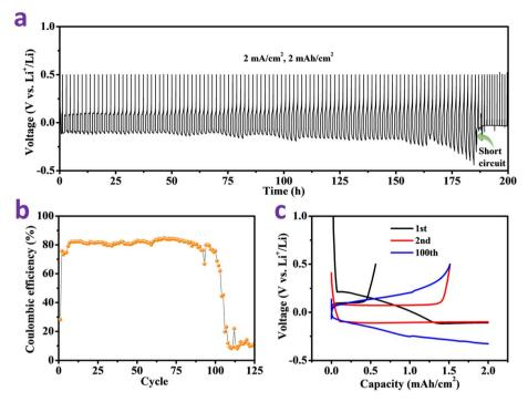
Fig. 3 (a) Cycling performance, (b) coulombic efficiency, and (c) corresponding voltage profiles of lithium plating/stripping on MnO<sub>2</sub>@Cu at a current density 2 mA cm<sup>-2</sup> and areal capacity of 2 mA h cm<sup>-2</sup>
