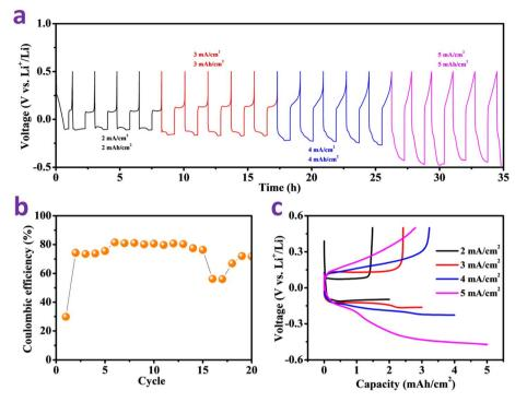
Fig. 6 (a) Rate performance, (b) coulombic efficiency, and (c) corresponding voltage profiles of lithium plating/stripping on MnO<sub>2</sub>@Cu at current densities of 2-5 mA cm<sup>-2</sup> and areal capacities of 2-5 mA h cm<sup>-2</sup>
