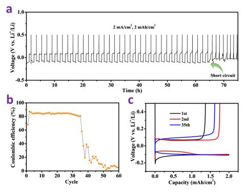
Fig. 2 (a) Cycling performance, (b) coulombic efficiency, and (c) corresponding voltage profiles of lithium plating/stripping on bare Cu at a current density of 2 mA cm<sup>-2</sup> and an areal capacity of 2 mA h cm<sup>-2</sup>.
