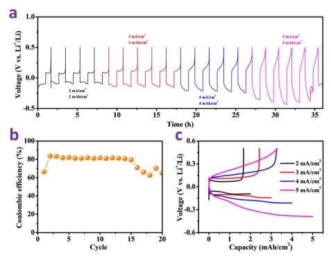
Fig. 5 (a) Rate performance, (b) coulombic efficiency, and (c) corresponding voltage profiles of lithium plating/stripping on bare Cu at current densities of 2-5 mA cm<sup>-2</sup> and areal capacities of 2-5 mA h cm<sup>-2</sup>.
