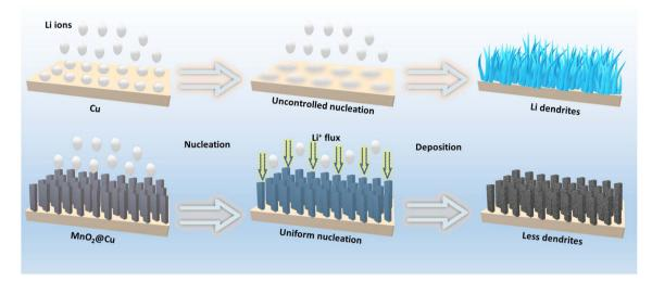
Lithium growth behavior during plating on bare Cu and MnO<sub>2</sub>-modified Cu current collectors
