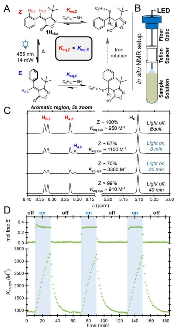
Fig. 3 (A) Equilibria involved in thiol-bonding and photoisomerization. (B) Diagram of the *in situ* LED NMR setup. (C) <sup>1</sup>H NMR spectra of **1H<sub>t</sub>Bu** equilibrated with OT without and during irradiation with 455 nm light. (D) Cycling experiment (455 nm irradiation for 20 min followed by a 40 min dark interval) for **1H<sub>t</sub>Bu** equilibrated with OT.
