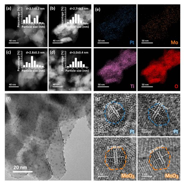
Fig. 1 HAADF-STEM images and corresponding particle size distributions of the (a) 6-Pt-MoO<sub>3</sub>, (b) 4-Pt-MoO<sub>3</sub>, (c) 2-Pt-MoO<sub>3</sub> and (d) 1-Pt-MoO<sub>3</sub> catalysts. (e) HAADF-STEM EDS mapping images, (f) TEM image and (g) HRTEM images of the 4-Pt-MoO<sub>3</sub> catalyst.
