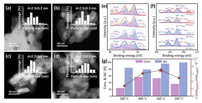
Fig. 5 HAADF-STEM images and corresponding particle size distributions of 4-Pt-MoO<sub>₹</sub> reduced at (a) 300, (b) 400, (c) 500 and (d) 600 °C. (e) Pt 4f and (f) Mo 3d XPS spectra of 4-Pt-MoO $_3$  catalysts reduced at various temperatures. (g) Catalytic performance of 4-Pt-MoO $_3$  catalysts reduced at various temperatures.
