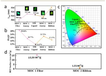
Fig. 8 (a) Influences of coordination and further assembly on solidstate emissions, corresponding (b) quantum yield and (c) CIE diagram, (d) specific surface areas of MOC 1-based nanofibers and MOC 2based micrometer ribbons.
