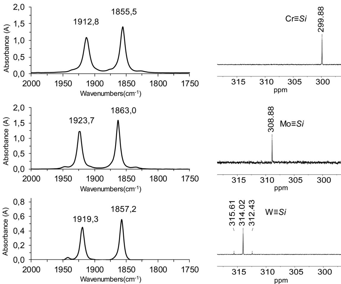
Fig. 5 (left) FT-IR spectra of the silyldiene complexes **1-Cr** – **1-W** in *n*-hexane in the spectral range 2000–1750  $\text{cm}^{-1}$  showing the two  $\nu(\text{CO})$  absorption bands; (right)  $^{29}\text{Si}\{^1\text{H}\}$  NMR spectra (99.36 MHz) of **1-Cr** – **1-W** in ( $D_6$ )benzene at 298 K showing the  $\text{M}\equiv\text{Si}$  signals.
