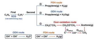
Fig. 2 Scheme of reaction routes during the CL-ODH process.
