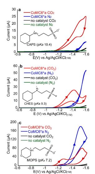
Fig. 3 CVs of 1  $\mu$ M CoMC6\*a in 50 mM (a) CAPS, (b) CHES, (c) MOPS. For all CVs, pH = 5.9, [KCl] = 0.1 M and scan rate = 100 mV s<sup>-1</sup>. Arrows in the CV traces indicate the scanning direction.
