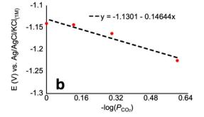
Fig. 5 (a) Linear sweep voltammograms of 1  $\mu$ M CoMC6\*a in 50 mM CHES, 0.1 M KCl, pH 5.9  $\pm$  0.1 at 100 mV s<sup>-1</sup> under different  $P_{\text{CO}_2}$ , the arrows indicate the direction of increasing  $P_{\text{CO}_2}$ . (b) Plot of  $E_i$  vs.  $-\log(P_{\text{CO}_2})$  showing a slope of  $\sim$ 150 mV per decade.  $R^2=0.94$ .
