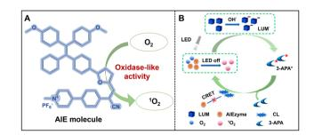
Fig. 2 (A) Illustration of AlEgens with enzyme-like activity; (B) possible mechanism for the sustained chemiluminescence of the AlEzyme/LUM system. Reproduced from ref. 59 with permission from American Chemical Society, copyright 2023.
