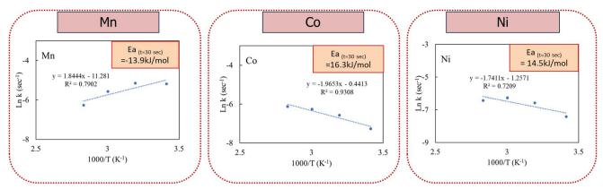
Fig. 8 Activation energy for Mn, Co, and Ni precipitation during the first 30 seconds of the reaction.
