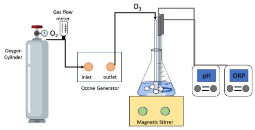
Fig. 1 Schematic experimental setup for ozone oxidative precipitation of Mn-Co-Ni from AMD
