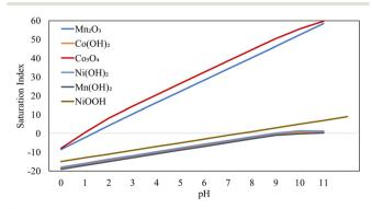
Fig. 2 Saturation indices of Mn-Co-Ni as a function of solution pH.
