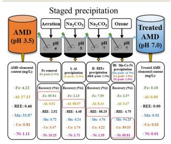
Fig. 10 Result of the integrated staged precipitation process developed for continuous AMD treatment at 150 mL min<sup>-1</sup> flow rate for Fe removal and selective recovery of Al, REEs, and Mn-Co-Ni.
