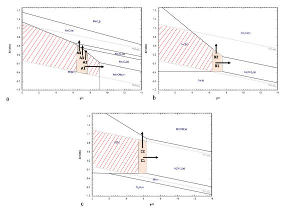
Fig. 3 Eh-pH diagrams for (a) Mn (1 mM), (b) Co (0.1 mM), and (c) Ni (0.1 mM), showing the predominant species in the H<sub>2</sub>O system at 25 °C.
