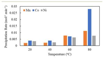
Fig. 7 Rate constant of Mn-Co-Ni precipitation at different temperatures (20, 40, 60, and 80 °C).
