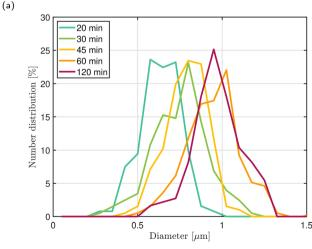
**Fig. 6** Evolution of the number crystal size distribution over time for MFI synthesized (a) under silent conditions and (b) under ultrasonication. All the curves are created from a minimum of 300 particles.
