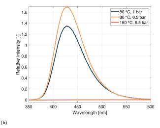
Fig. 4 Fluorescence spectra of 2-hydroxyterephthalic acid as a consequence of the interaction between terephthalic acid and radicals produced in the CR under different process conditions via (a) ultrasonication and (b) sodium persulfate as a radical initiator. All the curves have been normalized based on the intensity of the curve obtained from ultrasound-generated radicals at 25 °C and 1 bar.
