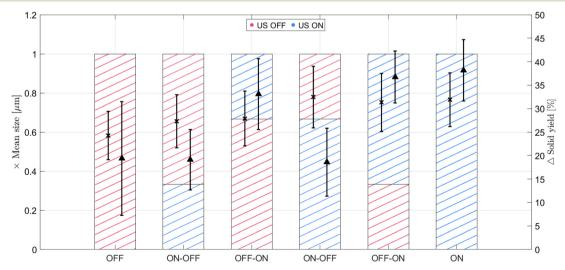
Fig. 8 Solid yield ( $\triangle$ ) and mean crystal size ( $\times$ ) for partial sonication experiment when 240 W power ultrasound (US) is applied for either 10 or 20 min on a total reaction time of 30 min, represented by the total height of the bar, and the top of the bar represents the end of the experiment.
