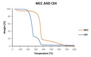
Fig. 7 Thermogravimetric profiles (TGA) of MCC and CE4.
