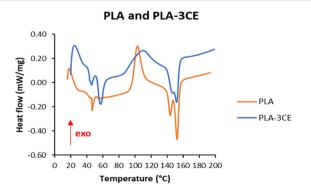
Fig. 8 DSC thermograms of PLA and the composite PLA-3CE.
