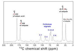
Fig. 3 The CP/MAS <sup>13</sup>C NMR spectrum of CE4, together with the structural assignments, indicated in red (adipate functionality) and blue (cellulose backbone).
