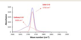
Fig. 2 Deconvolution of FT-IR spectrum of CE4 between 1600 and 1850 cm<sup>-1</sup>.
