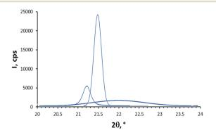
Fig. 6 Deconvolution of the XRD spectrum of CE4 in the  $2\theta$  range  $20-24^{\circ}$ .
