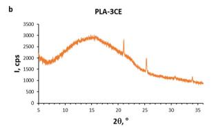
Fig. 9 XRD spectra of PLA (a) and the composite PLA-3CE (b).
