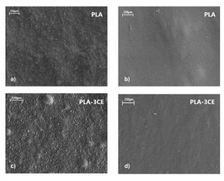
Fig. 10 SEM images of PLA and PLA-3CE film surfaces, exposed to air (a and c) and in contact with the Petri dish (b and d).
