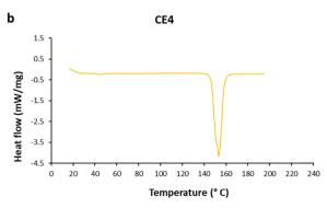
Fig. 4 DSC thermograms of MCC (a) and CE4 (b). First heating run, 10 °C min<sup>-1</sup>.
