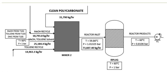
Fig. 3 PFD of the reactor step of the process.
