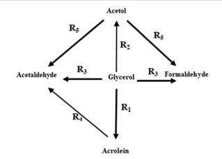
Fig. 3 The reaction pathway of the dehydration of glycerol over solid acid catalysts such as SiW<sub>20</sub>-Al/Zr<sub>10</sub> used in the CFD model. 10,11
