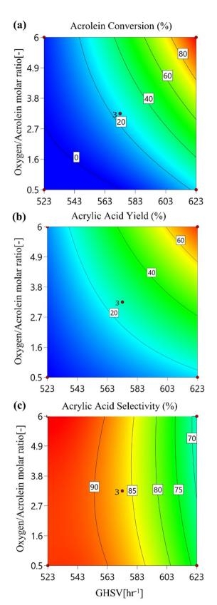
Fig. 12 Acrolein conversion (a), acrylic acid yield (b), and acrylic acid selectivity (c) versus reaction temperature at different oxygen/acrolein molar ratios (at 1 bar and a GHSV of 8800 h<sup>-1</sup>).
