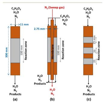
Fig. 1 Three simulated packed bed reactor schemes for the process of glycerol dehydration: (a): packed bed reactor (PBR), (b): sodalite membrane packed bed reactor (SMPBR), and (c): multi-bed packed reactor (MBPR).
