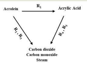
Fig. 4 Simplified scheme of the acrolein oxidation to acrylic acid on Mo-V-W-mixed oxides.
