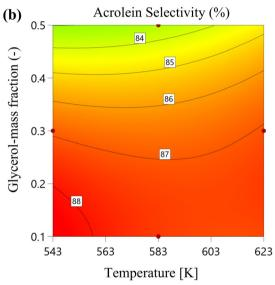
Fig. 8 Acrolein selectivity versus glycerol mass fraction at 1 bar reaction pressure: (a) by increasing reaction temperature and (b) by increasing GHSV value.
