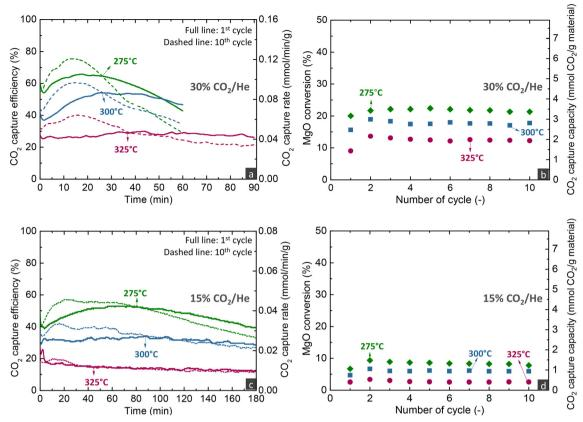
Fig. 6 (a) and (c) CO<sub>2</sub> capture efficiency and rate during the carbonation stage of the 1st and 10th cycles and (b) and (d) CO<sub>2</sub> capture capacity and MgO conversion over cycles for the MgCa<sub>0.05</sub>A<sub>0.20</sub> material when investigated via carbonate looping experiments in a fixed bed reactor with different temperatures and gas feeds for the carbonation stage (carbonation stage: 300 h<sup>-1</sup>; decarbonation stage: 450 °C, 100% He, 720 h<sup>-1</sup>).
