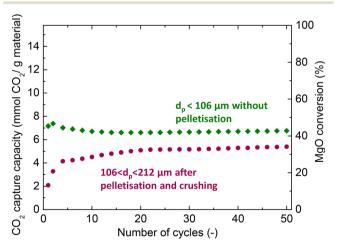
Fig. 2 CO<sub>2</sub> capture efficiency and MgO conversion for the  $MgCa_{0.05}A_{0.20}$  material obtained with and without pelletisation when investigated via carbonate looping experiments in a thermogravimetric analyser (carbonation stage: 30% CO<sub>2</sub>/N<sub>2</sub>, 300 °C; decarbonation stage: 450 °C, 100% N<sub>2</sub>).
