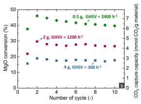
Fig. 5 (a) CO<sub>2</sub> capture efficiency during the carbonation stage of the 1st and 10th cycles and (b) CO<sub>2</sub> capture capacity and MgO conversion over cycles for the MgCa<sub>0.05</sub>A<sub>0.20</sub> material when investigated via carbonate looping experiments in a fixed bed reactor with different space velocities for the carbonation stage (carbonation stage: 30% CO<sub>2</sub>/He, 300 °C; decarbonation stage: 450 °C, 100% He, 720 h<sup>-1</sup>).
