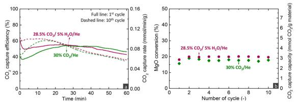
Fig. 7 (a) CO<sub>2</sub> capture efficiency and rate during the carbonation stage of the 1st and 10th cycles and (b) CO<sub>2</sub> capture capacity and MgO conversion over cycles for the MgCa<sub>0.05</sub>A<sub>0.20</sub> material when investigated via carbonate looping experiments in a fixed bed reactor under dry and wet operating conditions for the carbonation stage (carbonation stage: 300 h<sup>-1</sup>, decarbonation stage: 450 °C, 100% He, 720 h<sup>-1</sup>).
