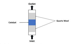
Fig. 3 Catalyst arrangement inside the reactor.
