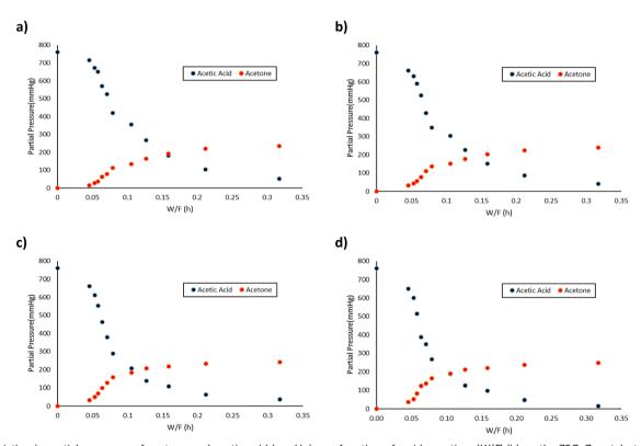
Fig. 7 Variation in partial pressures of acetone and acetic acid (mmHq) as a function of residence time (W/F) (h) on the 75CeZr catalyst (a: 300 °C, b: 325 °C, c: 350 °C, and d: 375 °C).
