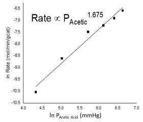
Fig. 5 Rate vs. partial pressure of acetic acid
