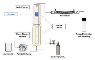
Fig. 2 Scheme for the experimental setup.
