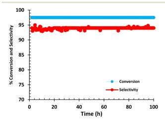
Fig. 11 Time on stream study. Reaction conditions: catalyst loading 2 g, reaction temperature 350  $^{\circ}$ C, and feed flow rate 0.1 ml min<sup>-1</sup>.
