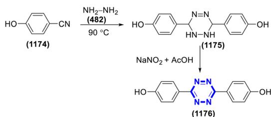
Scheme 326 Synthesis of tetrazines under catalyst-free conditions.
