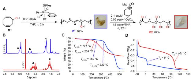
Fig. 2 (A). Reaction scheme and photographs for synthesis of P2. Representative <sup>1</sup>H NMR spectra (B), TGA (C), and DSC plots (D) for P1 (10 °C min<sup>-1</sup>;  $M_n = 86.7 \text{ kg mol}^{-1}$ ) and P2 (20 °C min<sup>-1</sup>). \*Equivalents calculated and reported relative to P1 repeat unit.
