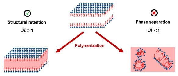
Fig. 6 The role of Artemis number, A, in successful polymerization in nanoconfinements.
