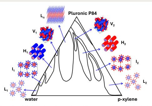
Typical phase diagram of water/oil/surfactant mixtures. Reproduced from ref. 63 with permission from American Chemical Society, copyright @1998.
