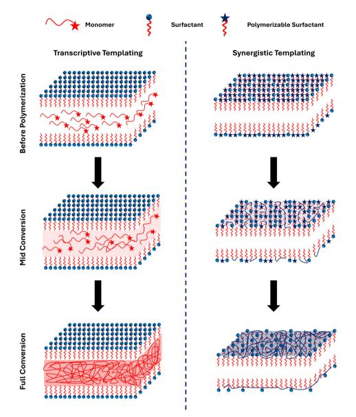
Schematic of LLC polymerization in transcriptive and synergistic templating methods.
