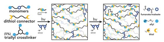
Fig. 9 Under first illumination, initial gelation from the polymer network occurs largely from thiol-ene addition and is advanced with slow chaingrowth homopolymerization. Over prolonged light exposure, the chain-growth homopolymerization forms additional crosslinks.
