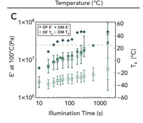
**Fig. 8** (A) DMA traces of DM network polymers illuminated for 30 s, 60 s, and 1800 s. (B) DMA traces of DF network polymers illuminated for 10 s, 60 s, and 1800 s. (C) E' at 100 °C and  $T_{\rm g}$  of DF and DM with error bars representing full width at half maximum of the glass transition. Collectively, these results suggest an increase in crosslinking density and network heterogeneity with continued light exposure.
