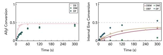
Fig. 5 <sup>1</sup>H NMR conversion of allyl (left) and maleate/fumarate (right) in 2:1 ratio\* photoreactions show a self-limiting reaction for DS, whereas combined maleate/fumarate and allyl consumption exceeds the number of available thiols. Combined with the observation of insoluble solids at long reaction times, this suggests some cross-reaction of allyls and maleates/fumarates is possible at low thiol concentration. \*The ratio is allyl: thiol or fumarate/maleate: thiol for DEF and DEM.
