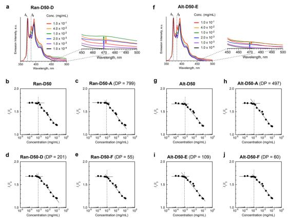
Fig. 5 CMC of amphiphilic random or alternating copolymers in water. (a and f) Emission spectra of pyrene  $(5 \times 10^{-7} \text{ M}: \text{normalized by } I_1)$  containing (a) Ran-D50-D and (f) Alt-D50-E in water. (b-e and g-j)  $I_1/I_3$  plots as a function of the polymer concentration  $(1.0 \times 10^{-4} - 1.0 \times 10^{-1} \text{ mg mL}^{-1})$  of (b) Ran-D50, (c) Ran-D50-A, (d) Ran-D50-D, (e) Ran-D50-F, (g) Alt-D50, (h) Alt-D50-E, and (j) Alt-D50-F.
