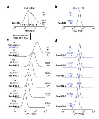
Fig. 2 SEC curves of Ran-D50 in (a) DMF (10 mM LiBr) and (b)  $\rm H_2O$  (100 mM NaCl) with PEO standard calibration. Ran-D50 was fractionated into six samples with different molecular weights (A–F) by preparative SEC. (c and d) SEC curves of fractionated Ran-D50-A–F with different DPs in (c) DMF (10 mM LiBr) and (d)  $\rm H_2O$  (100 mM NaCl). The  $M_n$  and D values are determined with PEO standard calibration.
