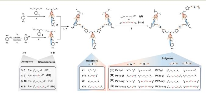
Scheme 1 The synthetic routes of target polymers and the corresponding structure characterization. Reaction conditions: (a) HCl (38%), NaNO<sub>2</sub>/H<sub>2</sub>O, CH<sub>3</sub>CN, 0-5 °C; (b) K<sub>2</sub>CO<sub>3</sub>, DMF, 80 °C; (c) DIAD PPh<sub>3</sub>, THF, 30 °C; (d) CuSO<sub>4</sub>·H<sub>2</sub>O, VcNa, THF/H<sub>2</sub>O, 30 °C; (e) NaN<sub>3</sub>, DMF, 80 °C; (f) CuSO<sub>4</sub>·H<sub>2</sub>O, VcNa, DMF, 25 °C.
