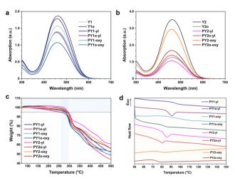
Fig. 3 (a) UV-vis spectra of monomers Y1 and Y1o and their corresponding polymers. (b) UV-vis spectra of monomers Y2 and Y2o and their corresponding polymers. (c) TGA thermograms and (d) DSC curves of polymers measured at a heating rate of 10 °C min<sup>-1</sup> under nitrogen.
