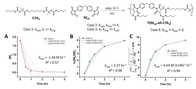
Fig. 1 Kinetic analysis of RAFT step-growth for maleimide monomers with the monomer M<sub>2B</sub> serving as a model monomer for fittings of various cases: (A) case 1, where  $k_{frag}$  is the rate-limiting step, (B) cases 2 and 3, where either  $k_{add}$  or  $k_{i}$  is the rate-limiting step, and (C) case 4, where all rate constants are equal.
