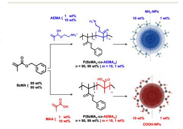
Fig. 1 Polymer synthesis scheme for P(BzMA-co-AEMA) and P(BzMA-co-MAA) and NP formation. The polymer's final composition was calculated based on mol% while the nomenclature is associated with the initial wt% of the monomers added.
