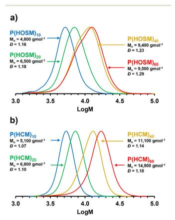
Fig. 5 Normalised GPC chromatograms for; (a) P(HOSM)<sub>x</sub> synthesised using column purified HOSM, and (b) P(HCM)<sub>x</sub> using brine washed HCM, by RAFT polymerisation in toluene at 70 °C targeting DPs of 10, 20, 40 and 60.
