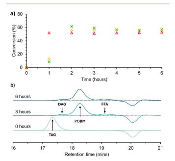
**Fig. 2** Data from the transesterification of HO-Sun oil; (a) conversion of glyceride bound fatty acids to POBMs vs. time at 30, 40 and 50 °C determined by  $^1$ H NMR spectroscopy, and (b) GPC chromatograms performed on 0, 3 and 6 h samples from the 30 °C experiment. Peaks have been labelled to highlight the most abundant species. FFA = free fatty acid, DAG = diglyceride, TAG = triglyceride, POBM = plant oil-based monomer.
