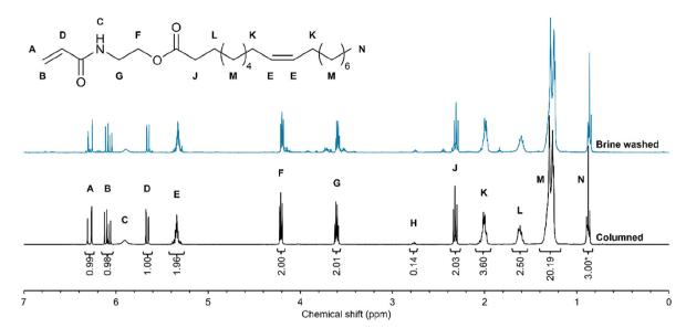
Fig. 3 <sup>1</sup>H NMR spectra (400 MHz, CDCl<sub>3</sub>, 25 °C) of the brine washed and column purified HOSM. Peaks for the column purified sample are assigned to the target structure and integrals (referenced against the CH<sub>3</sub> signal at 0.9 ppm) are displayed. Peak H corresponds to allylic protons from linoleic and linolenic FAs (structure not shown).
