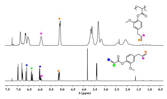
$\textbf{Fig. 4} \quad ^{1}\textbf{H NMR spectra (CDCl}_{3}, \textbf{RT): (top) P4aGA produced by the } \ DP^{f}\textbf{Bu}_{2}/B(2,4-F_{2}\textbf{C}_{6}\textbf{H}_{3})_{3} \ \textbf{FLP (Table 1, run 13); (bottom) 4aGA monomer. }$
