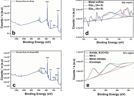
Fig. 2 (a) UV-Vis-NIR spectra of Au Ncap before and after Herceptin conjugation. XPS survey scan of (b) bare Au Ncap, and (c) Herceptin-functionalized Au Ncap. Deconvoluted XPS peaks of the (d) S 2p (e) N 1s regions for Herceptin-conjugated Au Ncap, respectively.
