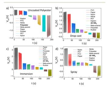
Fig. 3 Triboelectric series based on open-circuit voltage measurements over time for different triboelectric layers of TENGs tested with (a) uncoated polyester, (b) polyester coated with 2D WS<sub>2</sub> via drop casting, (c) polyester coated with 2D WS2 via immersion, and (d) polyester coated with 2D WS<sub>2</sub> via spray.
