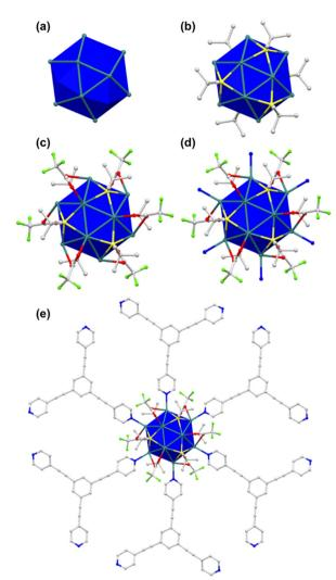
Fig. 3 Sequence of designing  $Ag_{12}$  cluster nodes and their connectivities in TUS 7: (a)  $Ag_{12}$  cluster core stabilized by (b) six  $-S^tBu$  ligands and (c) six  $-CF_3COO$  ligands. (d) N sites and (e) the corresponding organic linkers coordinated to the  $Ag_{12}$  nodes. H atoms are removed for clarity.
