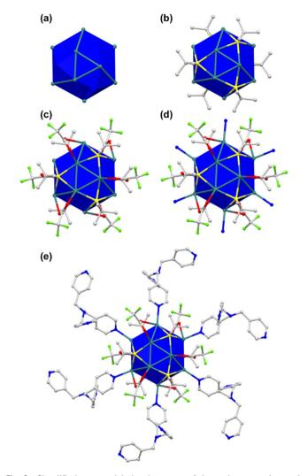
Fig. 2 Simplified sequential development of  $Ag_{12}$  cluster nodes and their connectivities in TUS 6: (a) cluster core comprising 12 Ag atoms and protected by (b) six -S<sup>t</sup>Bu ligands and (c) six -CF<sub>3</sub>COO ligands. (d) N sites and (e) the corresponding organic linkers coordinated to the Ag<sub>12</sub> nodes. H atoms are removed for clarity.
