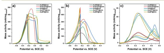
Fig. 7 Mass activity of different types of multimetallic nanoparticle electrodes in the MOR (a), EOR (b) and FAOR (c). The total metal concentration was kept constant during the preparation of all electrodes.
