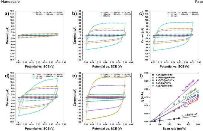
Fig. 6 Scan rate dependent CV curves of GCE electrodes modified by multimetallic nanoparticles with spherical (a), prism-shaped (b), octahedral (c), rod-shaped (d), and bipyramidal (e) cores in 1 M KOH electrolyte. Double layer capacitances for the different types of multimetallic nanoparticle electrodes (f).
