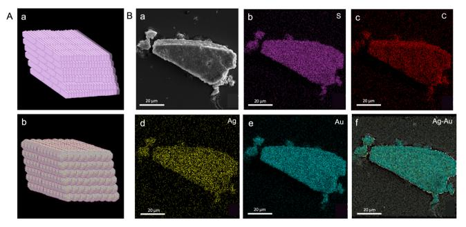
Fig. 3 (A) Schematic illustration of a slanted cuboidal-shaped mesocrystal (a) and its compositional representation (b). (B) FESEM image of such a crystalline entity (a) and the corresponding EDS maps of S (b), C (c), Ag (d), Au (e), and Ag-Au overlay (f). Illustrations are created with a licensed version of BioRender.com.
