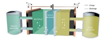
Fig. 12 Schematic of the reversible redox reaction of Zn and V in the Zn-V flow battery. 63 Copyright 2023, the American Chemical Society.
