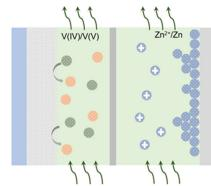
Fig. 1 Schematic of the static Zn-V battery (vanadium-based zinc-ion batteries) and Zn-V flow battery.
