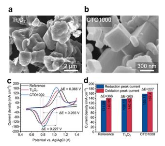
Fig. 16 SEM images of (a) Ti<sub>4</sub>O<sub>7</sub> and (b) CTO1000 electrocatalyst. (c) Cyclic voltammograms of pristine CF, Ti<sub>4</sub>O<sub>7</sub>, and CTO1000 electrodes. (d) Reduction and oxidation peak currents and potential difference of pristine CF, Ti<sub>4</sub>O<sub>7</sub>, and CTO1000 electrodes.<sup>63</sup> Copyright 2023, the American Chemical Society.
