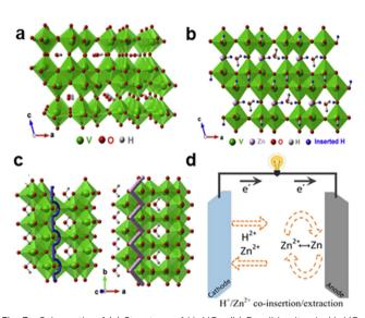
Fig. 3 Schematic of (a) Structure of H-VO<sub>2</sub>. (b) Possible sites in H-VO<sub>2</sub> for H<sup>+</sup>/Zn<sup>2+</sup> co-intercalation/extraction. (c) Migration pathways for H<sup>+</sup> (left) and  $Zn^{2+}$  (right) ions in H-VO<sub>2</sub>.8 Copyright 2020, Elsevier. (d)  $H^+/$ Zn<sup>2+</sup> co-intercalation/extraction mechanism in static Zn-V batteries (vanadium-based zinc-ion batteries). 6 Copyright 2021, Elsevier.
