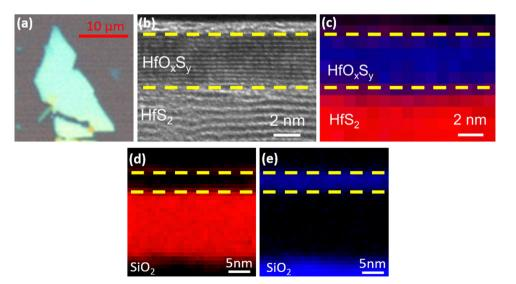
Fig. 1 (a) Optical microscopy image of HfO<sub>x</sub>S<sub>v</sub>/HfS<sub>2</sub> flakes before being transferred to lamella for transmission electron microscopy (TEM). (b) Crosssectional TEM image of partially oxidised flake shows crystallinity of the resulting oxide layer and (c) electron energy-loss spectroscopy (EELS) mapping of (d) sulfur (red) and (e) oxygen (blue) demonstrates a clear separation of the  $HfO_xS_v$  and  $HfS_2$  regions.
