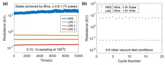
Fig. 3 (a) Non-volatile states achieved by 80 ns pulse programming are retained over 10<sup>4</sup> s at 150 °C. (b) Pulsed voltage resistance switching unaffected by operating device in an 8.6 mbar vacuum environment.
