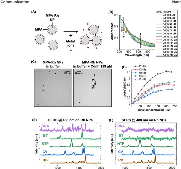
Fig. 3 (A) Sketch of the MPA-Rh NP optical sensor based on the coordination of metal ions by the carboxylic groups of MPA. (B) Evolution of the optical spectra of MPA-Rh NPs while increasing the concentration of Cd(II). (C) TEM images of the MPA-Rh NPs before and after the addition of Cd(II). (D) Response of the optical sensor for different metal ions. (E) and (F) SERS spectra of bare Rh NPs excited at 458 nm (E) and 488 nm (F).
