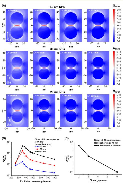
Fig. 6 (A) Bidimensional maps of the  $G_{SERS}$  in the equatorial plane of Rh NP dimers with a gap of 2 nm and sizes of 20, 30 and 40 nm excited at 350, 458, 488 and 633 nm in a medium with refractive index n = 1.334. (B) Plot of the  $G_{SERS}$  maximum versus the excitation wavelength for the three dimer sizes considered. (C) The plot of the  $G_{SERS}$  maximum versus the gap size for an excitation wavelength of 350 nm and dimers with a size of 40 nm.
