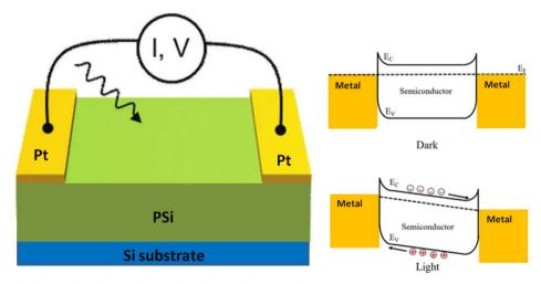
Energy bandgap diagram of the Pt/PSi/Pt device.
