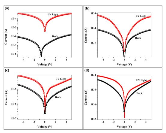
Fig. 9 I-V characteristics of the designed photodetectors based on n-PSi films annealed at (a) 3, (b) 5, (c) 10, and (d) 20 laser pulses recorded under dark and UV light conditions.
