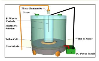
Fig. 1 Graphical representation of the PECE cell used to generate n-PSi samples.
