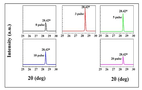
XRD patterns of the n-PSi samples annealed under varying laser pulses.
