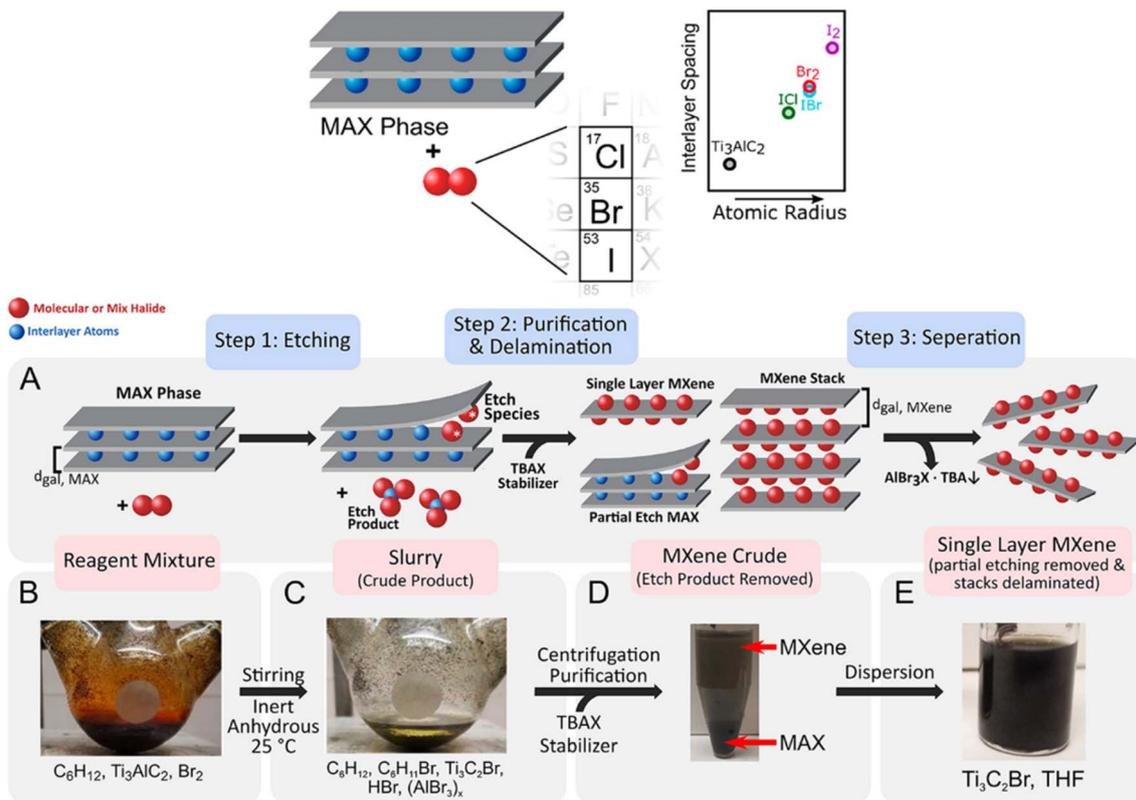
Fig. 2 (A–E) Halogen etching of Ti<sub>3</sub>AlC<sub>2</sub> MAX phase. Reproduced from ref. 48 with permission from American Chemical Society, copyright 2021.
