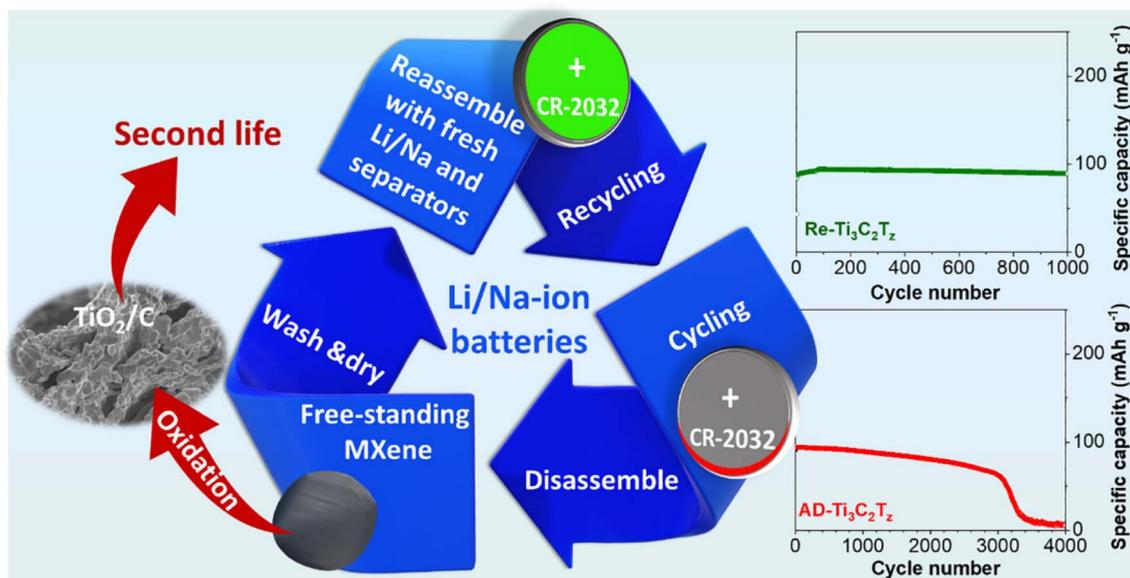
Fig. 10 Second life of Ti<sub>3</sub>C<sub>2</sub>T<sub>x</sub> electrodes for LIBs/SIBs. Reproduced from ref. 78 with permission from Elsevier, copyright 2023.
