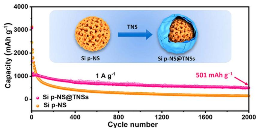
Fig. 8 Interfacial assembly  $\text{Ti}_3\text{C}_2\text{T}_x/\text{Si}$  for the enhancement of electrochemical Li storage activity. Reproduced from ref. 73 with permission from the American Chemical Society, copyright 2020.
