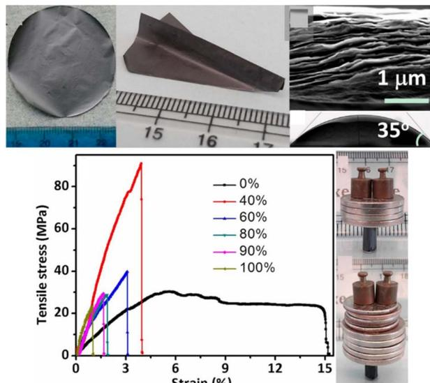
Fig. 4 Mechanical properties of a metallic  $\text{Ti}_3\text{C}_2\text{T}_x$  MXene film. Reproduced from ref. 61 with permission from the National Academy of Sciences of the United States of America, copyright 2014.
