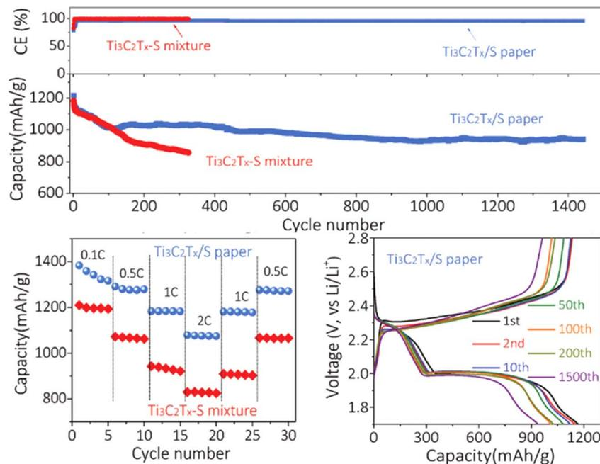
Fig. 9 Cycling properties, rate capability, and charge–discharge profiles of the S@Ti<sub>3</sub>C<sub>2</sub>T<sub>x</sub> composite. Reproduced from ref. 77 with permission from John Wiley and Sons, copyright 2019.
