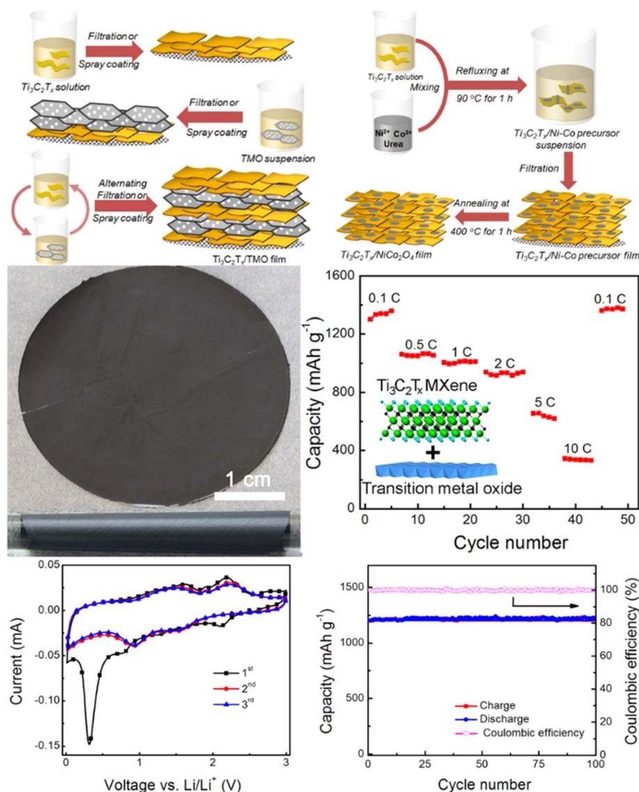
Fig. 11 Schematic illustration of the combination of  $\text{Ti}_3\text{C}_2\text{T}_x$  MXene with transition metal oxide to obtain hybrid electrodes for energy storage. Reproduced from ref. 81 with permission from Elsevier, copyright 2016.
