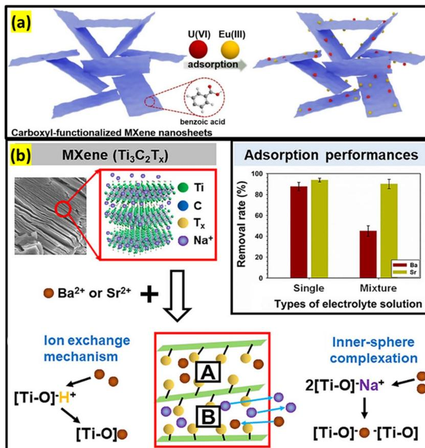
Fig. 14 Carboxyl-functionalized  $\text{Ti}_3\text{C}_2\text{T}_x$  nanosheets (a) for the removal of U(vi) and Eu(III), and (b) for treatment of  $\text{Ba}^{2+}$  and  $\text{Sr}^{2+}$ . Reproduced from ref. 114 and 115 with permission from Elsevier, copyright 2020.
