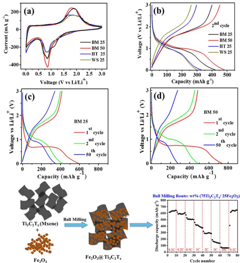
Fig. 7 (a–d) Effect of preparation on the performance of  $\text{Fe}_2\text{O}_3/\text{Ti}_3\text{C}_2\text{T}_x$  anode materials for LIBs. Reproduced from ref. 71 with permission from American Chemical Society, copyright 2018.
