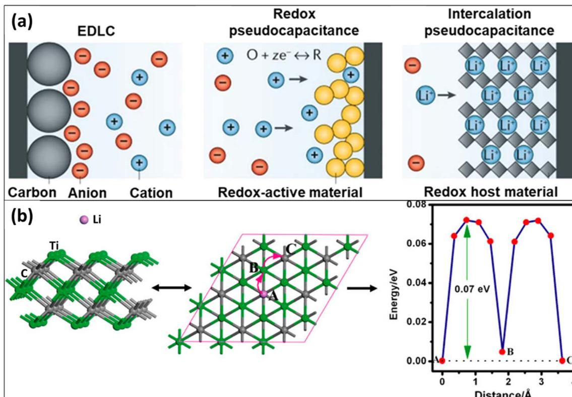
Fig. 5 Schematic illustrations depicting (a) the mechanisms of electrochemical charge storage and (b) the pathways for lithium diffusion within  $\text{Ti}_3\text{C}_2\text{T}_x$  MXene. Reproduced from ref. 66 with permission from Springer Nature, copyright 2019. Reproduced from ref. 65 with permission from the American Chemical Society, copyright 2012.
