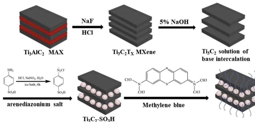
Fig. 15  $\text{Ti}_3\text{C}_2\text{T}_x$ - $\text{SO}_3\text{H}$  composite for the removal of methylene blue in an alkaline environment. Reproduced from ref. 120 with permission from Elsevier, copyright 2019.
