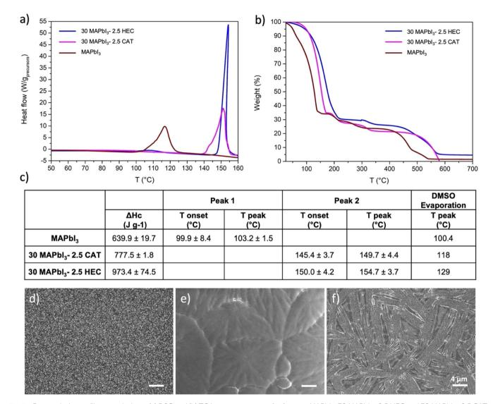
From solution to film morphology. (a) DSC and (b) TGA measurements of reference MAPbl<sub>3</sub>, 30 MAPbl<sub>3</sub>–2.5 HEC and 30 MAPbl<sub>3</sub>–2.5 CAT, along (c) values extracted from TGA; SEM analysis of (d) reference MAPbl<sub>3</sub>, (e) 30 MAPbl<sub>3</sub>-2.5 HEC and (f) 30 MAPbl<sub>3</sub>-2.5 CAT, scale bar: 4 µm.
