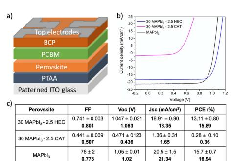
Fig. 4 Photovoltaic parameters of the PPnc based PSCs. (a) p-i-n Device architecture and (b) characteristics J-V of the best device based on 30 MAPbl<sub>3</sub> - 2.5 HEC, 30 MAPbl<sub>3</sub> - 2.5 CAT and reference MAPbl<sub>3</sub>. (c) Average values (on 30 devices) and best performance (bold font).
