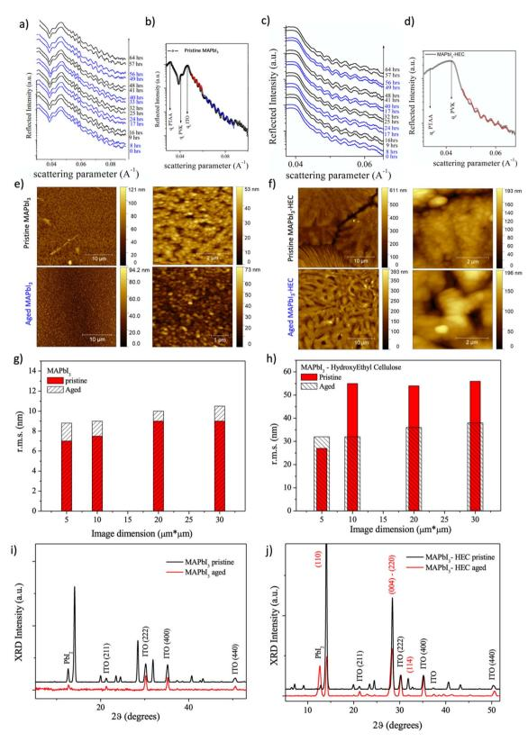
Fig. 5 EDXR, AFM and XRD characterization. EDXR measurements during dark-light cycles for (a and b) reference MAPbI<sub>3</sub> and (c and d) 30  $MAPbl_3 - 2.5 HEC$ ; AFM analysis on (e) Reference  $MAPbl_3$  and (f) 30  $MAPbl_3 - 2.5 HEC$ , of pristine (top row) and aged (bottom row) samples, with relative (g and h) rms evaluation; XRD patterns of (i) reference MAPbl<sub>3</sub> and (j) 30 MAPbl<sub>3</sub> - 2.5 HEC before and after the aging process.
